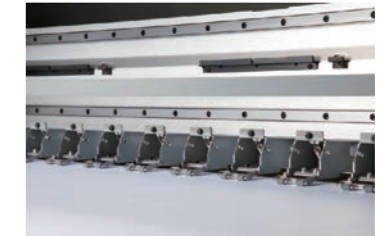
Newly designed pinch rollers
